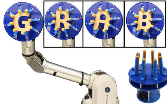
Fig. 1. The proposed 8-finger single-actuator fixturing gripper mounted on a robot arm and grasping planar lamina. Each finger translates radially inward until it comes in contact and exerts the same force on the lamina. Upon contact, the fingers lock passively and create a form closure grasp.
