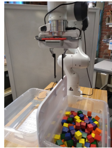
Fig. 4. Franka Emika Panda setup with adapted fingertips.
