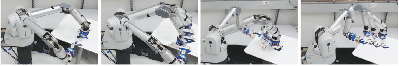
Fig. 8. Real executions of the proposed planner using a WAM arm installed with a Yale T42 hand. The objects are perceived using a Kinect sensor installed over the tabletop. The plastic “Y”, “A”, “L” and “E” letters are grasped after executing the pre-grasp top-sliding manipulations planned by our planner. More example executions can be found in the supplementary video.
