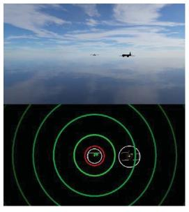
The simulated airspace is given a realistic background and contains moving obstacle aircraft.
